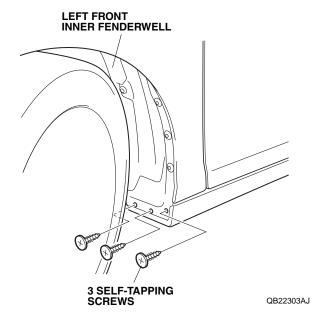
4. Install the left front splash guard to the left front inner fender with one self-tapping screw supplied, and the three self-tapping screws removed in step 3 in this order 1→2→3→4. Check that there is no gap between the left front splash guard and the vehicle body. If there is a gap, loosen the four self-tapping screws, hold the splash guard against the body, and retighten the screws.
