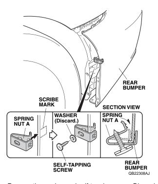
10. Remove the washer and self-tapping screw. Discard the washer, it will not be reused.
